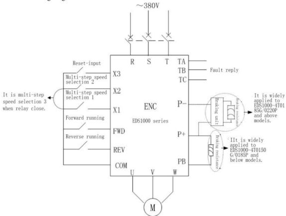
当继电器同时闭合为多段速选择 3: It is multi-step speed selection 3 when relay close.
